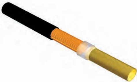
Wire is stripped and the appropriate size crimp sleeve is slid onto the strands.
