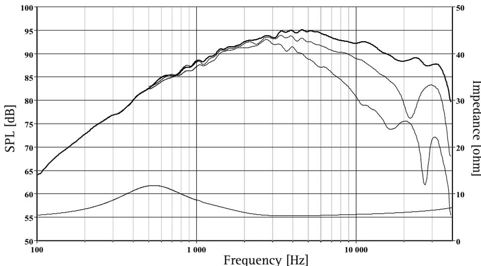
The frequency responses above show measured free field sound pressure in 0, 30, and 60 degrees, mounted in a 0.6m by 0.8m baffle. Input 2.83 V<sub>RMS</sub>, microphone distance 0.5m, normalized to SPL 1m. The impedance is measured without baffle using a 2V sine signal.
