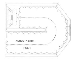
Transmission line enclosures should be completely filled with Acousta-Stuf fiber from just behind the woofer, all the way down the length of the line to the terminus opening. This usually requires between 1/2 and 1 1/2 pounds per cubic foot of enclosure.
