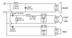
This is an another 3-way example switching the horn to H400 and super tweeter to T900A. Network's basic design is the same but crossover frequency between super tweeter and midrange is changed to 7kHz.
