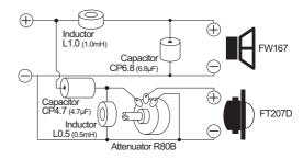
Example of FW167/FT207D, 2 way standard bass reflex type enclosure. Internal volume is 20 liters tuned to approximately 43Hz (Fb). Model 'R80B' attenuator is also used for varying tweeter level.
