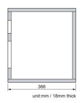
This is an example of 2 way system using FW167/FT207D with the closed type enclosure. Internal volume is 30 liters. The same network as above bass reflex example can work properly.
