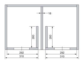
This is an example of sub-woofer system using FW167 x 2pcs with bass reflex type enclosure. Each cavity's internal volume is approx. 23 liters and tuned to 49Hz (Fb). Installing terminal for each, it can be driven L/R independently or center sub-woofer  $(4\Omega)$  with wired in parallel.
