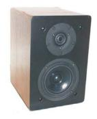
The Studio is a small monitor type speaker using the new Vifa XT ring radiator tweeter and the Vifa Premium Line 5" woofer. A 6" passive radiator is used on the back to tune the enclosure and extend the bass response. The frequency range is from 45Hz to 20kHz with very impressive bass for such a small
