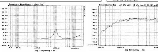
Measured on IEC baffle using Bruel & Kjaer 3144 model microphone. Sensitivity Mag at 0, 30, and 45 deg.
